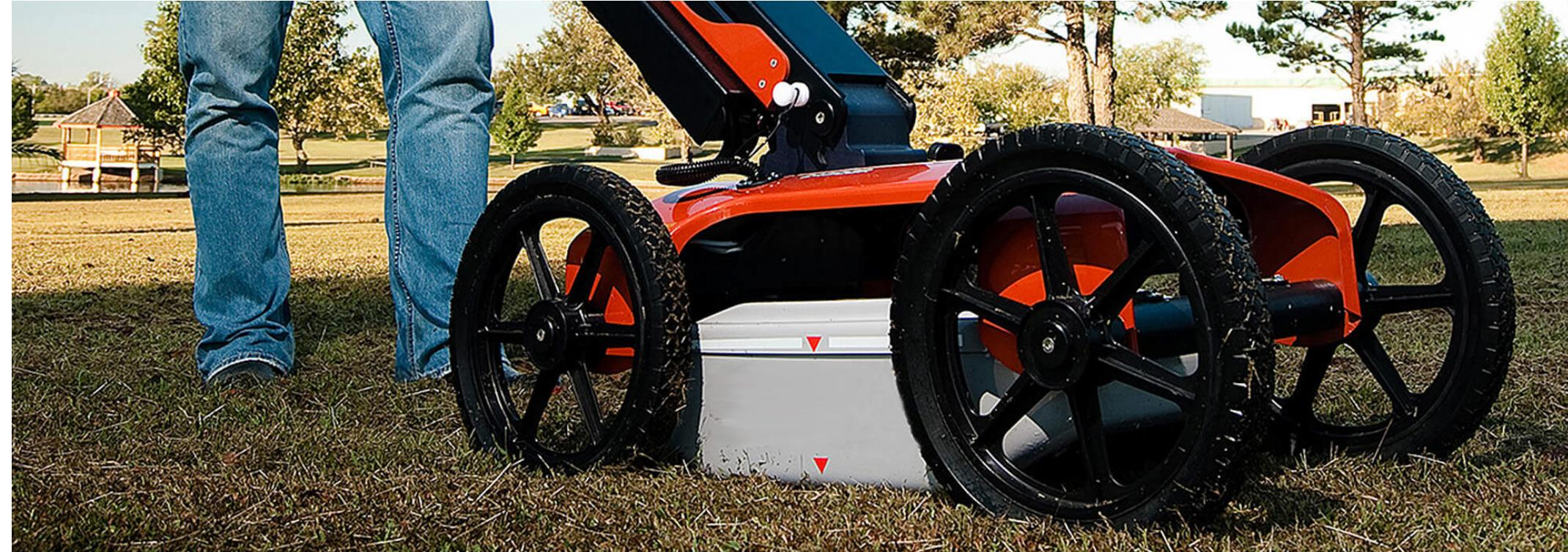
**Ground Penetrating Radar:** Ground Penetrating Radar (GPR) helps identify the location of underground utilities. A device that looks similar to a lawnmower, and is nondestructive to the soil, uses radio frequencies to detect objects below the ground's surface. Maps and images are created from the data.
